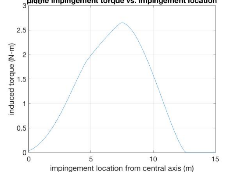
plume impingement torque vs. impingement location
